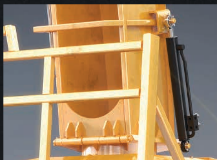
Throwing tube is turning into transport position by 2 cylinders
